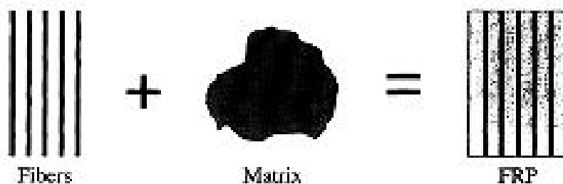
Figure 1: Formation of fiber reinforced polymer composite
